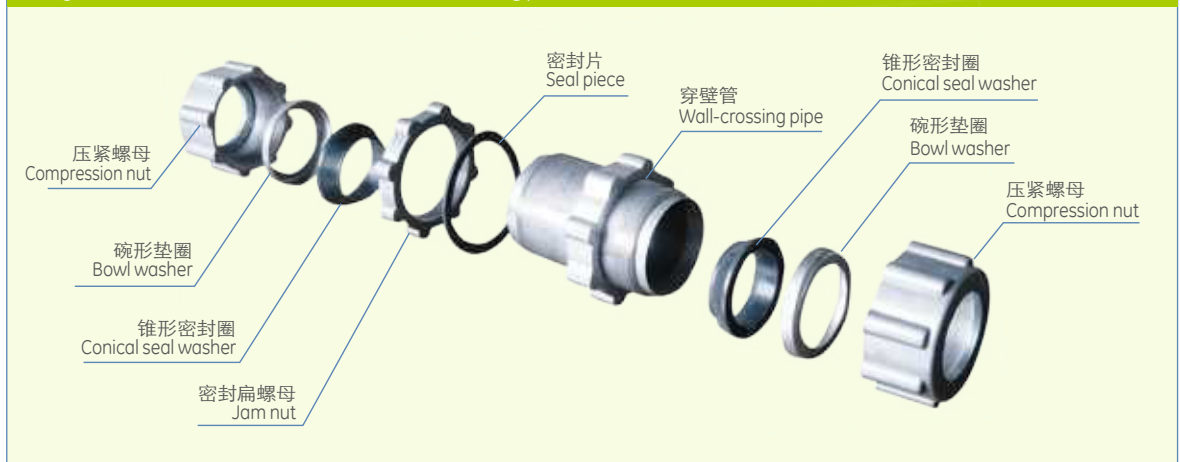
Fig.2. Structure of FAP-A-2 dual end type
